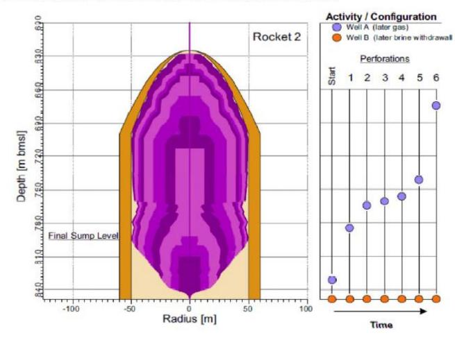
Dual Well Configuration: Platform wireline perforations avoids need for costly drill rig.
