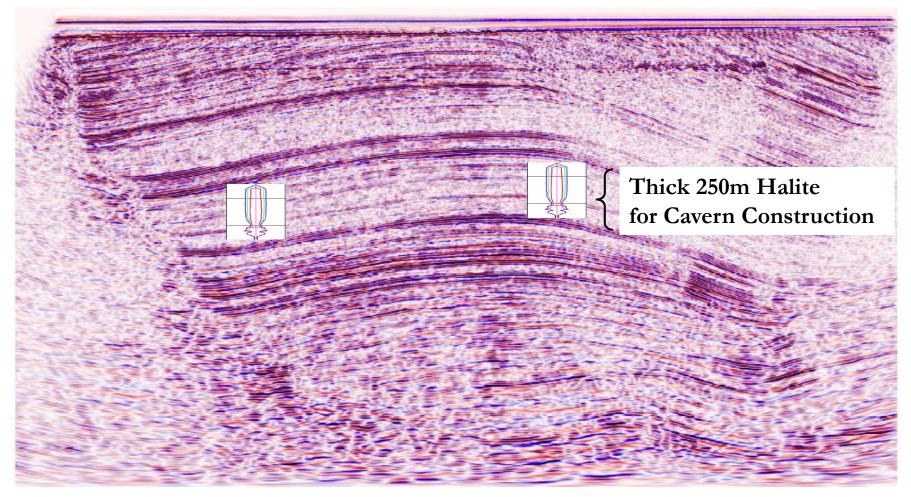
Example UHR seismic line:
